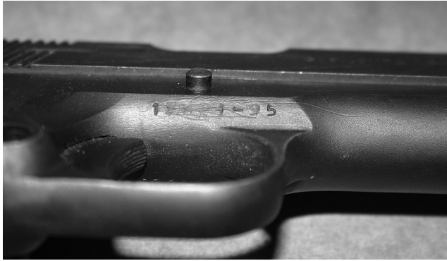
Figure 5.5 A scratching type attack on a pistol. As can be seen, the obliteration was only partial, and the number was restored chemically with relative ease. (Image from author's collection.)
